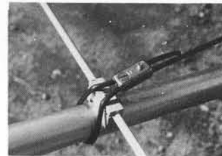
Mounting of guy wire on boom
